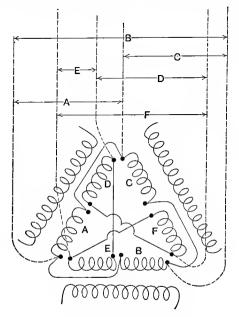
FIG. 106. Transformer connections for three-phase, six-phase transformation.
